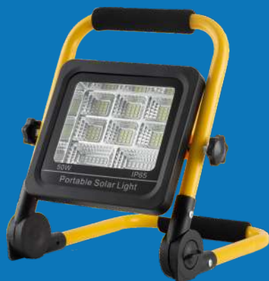
FL33/RCH/LED/50W (8859) PORTABLE SOLAR RECHARGEABLE LED FLOOD LIGHT 50W, H270XW235XD50MM, IP65, ABS+Glass Multi-functional, USB & Solar Charging+Power Bank Integrated Solar Panel, Li-ion Batteries and USB Cable included Four Gear Working Mode (100%, 50%, 20% & Flashing) Charging time: 6H, Working time: 15-30H
