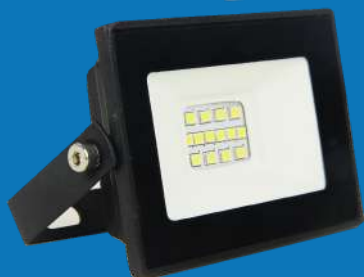
FL30 ECONOMIC DRIVERLESS LED FLOOD LIGHTS 10W TO 100W IP65, Aluminium+Tempered Glass
